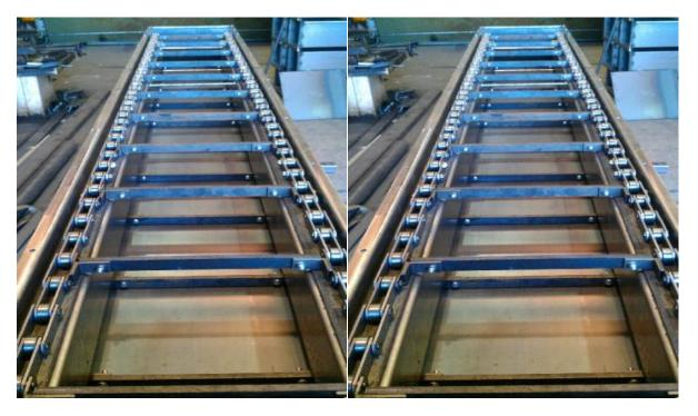
Each component is made from high-quality steels and then specially heat-treated to provide maximum performance and long wear life. Joint parts are hardened to provide greater strength and wear resistance. Sidebars are hardened to achieve ultra-high strength throughout.
