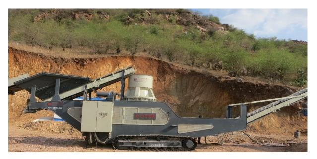
Conmix Cone Crusher range of mobile cone crushers are suitable for secondary and tertiary crushing in direct feed applications. The range uses advanced Track Mounted Cone Crusher is to provide high volumes of excellently shaped product In Ahmedabad, India.
