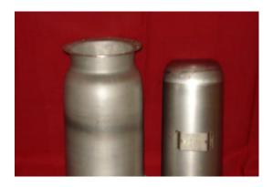
We manufacture geyser inner steel from capacities 1 Liter, 3 Litres & 6 Litres. Postfinishing operations such as project arc welding, necking , multihole punching, Polishing and Buffing operations are also being carried out.
