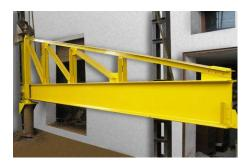
Eagle make Jib Cranes have large heights and large boom length. Special foundation is carried out for this type of crane to withstand the unique technical specifications. These cranes are having 90° - 360° rotation. These rotation is manually as well as electrically.
