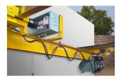
Eagle manufactures Single Girder as well as Double Girder cranes in the Underslung version. Such cranes find applications where the headrooms available are limited or the process requirements cannot allow any other means of supporting the crane except from the roof.
