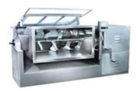
The mass mixer consists of a rigid fabricated structure motor, gear box, mixing drum, stirrer and tilting device. Specially designed self adjusting sealing arrangement of unique design is provided to ensure that no black particle enters into the mixing drum. The material under mixing process can be monitoring through acrylic dust cover and its controls dusting and contaminations. The tilting device is provided to make easy the unloading of the material and easy cleaning of the mixing drum.
