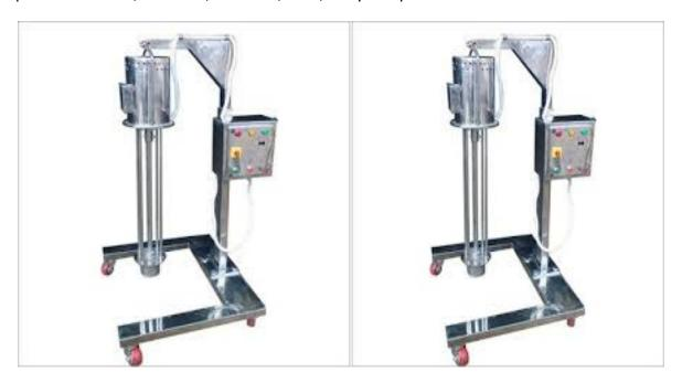
This machine is used for mixing, blending, dispersion, homogenization and emulsification of liquids, paste, ointment, solution, viscous material and solids into other liquids. This machine consists of specially designed rotor and stator assembly, fixed with four tie rods to the motor. This rotor rotates inside the stator assembly and thus reduces the particle size of the droplets and also reduces batch time.
