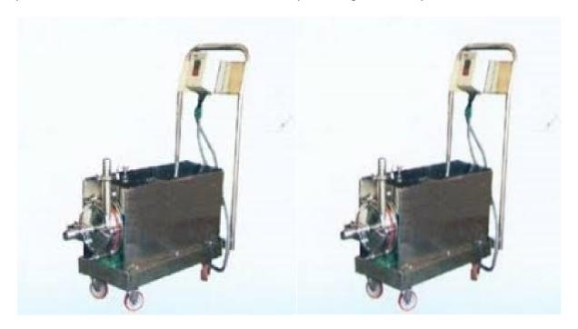
The machine is made compact and versatile, having a SS make gear pump coupled with an electric motor or an electric geared motor. Whole unit is mounted on a SS Trolley provided with castor wheels. The rigid design of the SS made gears and houses allows high pressures and the ability to pump highly viscous fluids. The material enters from inlet of the pump, the meshing of the gears displaces it forward, and then it got discharged from the outlet of the pump.
