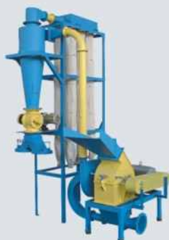
Simple Pneumatic Conveying System
