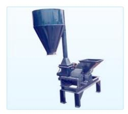
An extra heavily constructed machine designed to pulverize even rocks & minerals of medium hardness. Fineness ranging between 100 mesh to 300 mesh (150 to 50 microns) and in some cases upto 500 mesh. "Non concrete foundation "frame with AVM pads may be provided.
