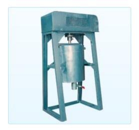
We fabricate Attritor Mills which are also known as Stirred Mills and are manufactured from superior grade steel that incorporates high efficiency in the machine. These are used in grinding and blending process for wet or dry materials. Our product range is equipped with a top cover that can be used to lock the main vessel with following features:
