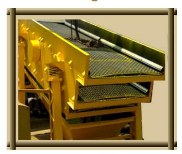
The Vibrating Screen is use for Separation of material in various size (as per your requirement). The rotary screen and vibrating screen are use in same purpose. However, in higher capacity and accuracy of product material the vibrating screen is necessary. The vibrating screen is normally manufactured one deck to five decks and the size is depending on capacity of per hour.
