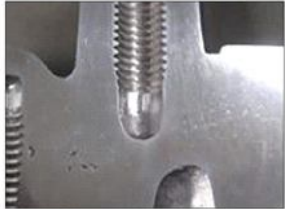
Casting when using Jet Cool System (Porosity decreases)
