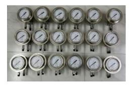
A Differential Pressure Gauge works on the pressure difference acting on the sensor, bourbon or diaphragm or on both sides ( h. P & I. P ) of a cylinder which gets a displacement that actuates a gear movement or any similar mechanism to an indicating pointer which moves over a dial marked in difference of pressure.
