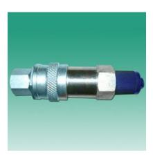
The arrangement as shown acts as a self acuating coupler. The valve is spring loaded and normally it keeps the valve pressured against the seat, thus remains closed when the pressure gauge pushed to the coupler the valve remain pressed against spring thus opening the seat & clears the air passage to pressure gauge which will be in operation. Air passed stop on removing the gauge.
