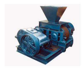
Fine grains of Coal/Coke or Charcoal mixed with suitable binder fed into the nip of a pair of counter rotating rolls and are compacted in mass of uniform shape and size, called briquettes. The separating force during the process is resisted by mechanically by 2 nos pressure bolts.
