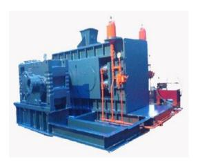
Fine grains of Coal/Coke/Charcoal/Ores and Minerals mixed with suitable binder fed into the nip of a pair of counter rotating rolls and are compacted in mass of uniform shape and size, called briquettes. The separating force during the process is resisted by suitable Hydraulic System equipped with Cylinders, Power-Pack or Hand Pump and Nitrogen Accumulator to absorb momentary shocks.
