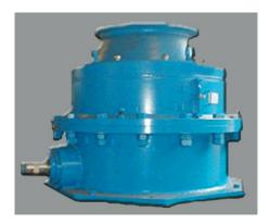
Cone crushers are used for crushing of medium-hard to extremely hard, tenacious and brittle products demanding a final grain with a high cubic grain proportion. The lower part of the housing includes the hydraulic piston for gap adjustment, the upper section accommodates the crushing zone. Crushing of the feed material is effected between the eccentrically rotating crushing cone and the fixed crushing shell.
