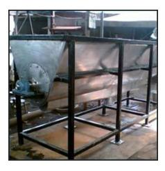
The Screw Conveyor is of simple design, of small width, permits intermediate discharge of the material at several points (of special importance for dusty, hot materials and materials with an obnoxious odour), is dust-tight by jacketing the trough.
