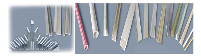
The very nature of Fiberglass, allow it to be used as an alternative to steel. It is very easy to assemble and can be cut, moulded, etc. as per specifications. The "FibrTuf" structural profiles are a combination of fiberglass reinforcements and thermosetting polyester or vinyl ester resin systems. It is produced in 51 varieties / plateholder / standard shapes.
