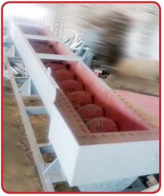
solids to settle out, whereupon they are removed by mechanical means. Solids that do not settle report as overflow from the pool. Up gradation of 2 to 3% is achieved improving qualities of end product. We offer wide range of spiral classifier, industrial spiral classifier, industrial spiral separator, solid liquid separators and spiral separator.
