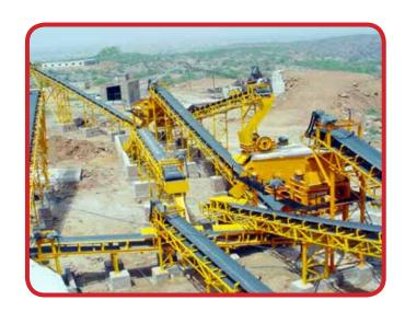
Works manufactured conveyor frame in 24", 30", 36", 42", 48" & 52" width by different size of channels.
