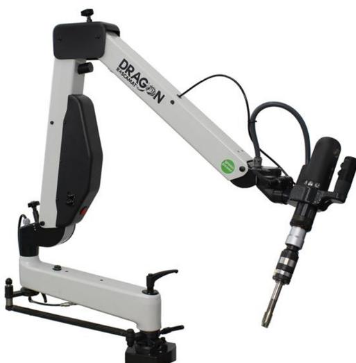
The machine consist of a radial supporting both articulated arms that can be adjusted by means of hte regulation handwheels to position them at the operator's convenience
