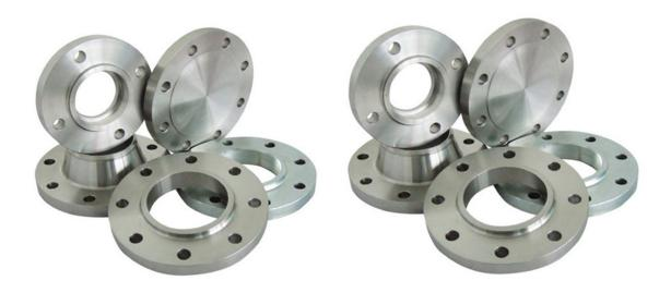
A flange is a method of connecting pipes, valves, pumps and other equipment to form a piping system. It also provides easy access for cleaning, inspection or modification. Flanges are usually welded or screwed. Flanged joints are made by bolting together two flanges with a gasket between them to provide a seal.
