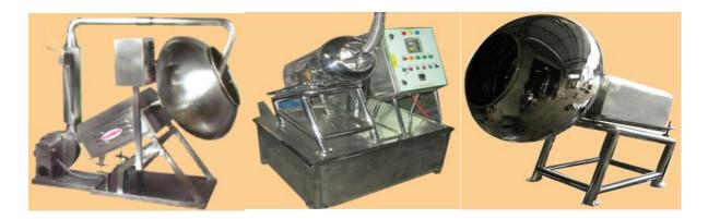
Coating Pan is made after a careful study of the needs of expert coaters such as Rotational Speed, Angle of inclination of Pan, Volume and Temperature. It is elliptical in shape, mounted at 30° angle. We also make available Coating Pan in other geometrical shapes and mounting angles, as per the requirement. RPM of the pan is variable. Hot air blower thermostat of the pan delivers required quantity of air at selected temperatures between 40°C to 80°C.
