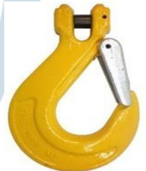
Clevis Hook Alloy Steel Gr. 70 Chain Size 1/4" to 3/4" Capacity 1.0 Ton to 10.0 Ton
