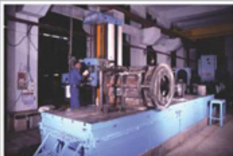
Spanish Make 6.5 m Bed CNC Floor Borer
