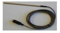
Thermowell is used to sense the temperature of the reaction medium inside the Autoclave.
