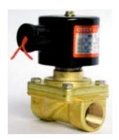
Either Solenoid Valve (FLP, IIC) or pneumatically actuated Ball Valves can be used. These valves are connected at the inlet of the internal cooling coil with external source of cooling water supply. Normal tap water is not preferable as it does not give effective cooling at higher temperatures due to steam back pressure.
