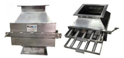
Drawer magnets consists of a row, or most commonly, rows of round magnetic tubes that are assembled into drawers. Drawer Magnets are recommended for fine cohesive materials such as magnesium oxide, zircon powder, fly ash, aluminum, gypsum, lime, powdered sugar, cornstarch, flour & pulverized minerals and ceramics.
