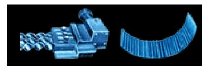
Rotor Shaft Assembly is a mild steel shaft fitted with plates and set of Forged Alloy steel Beaters [Hammers] of Rotor shaft assembly, evolving at high velocity in the grinding chamber and beating the materials as it enters from the screw feeders.
