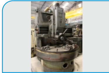
Russian VTL Sedin 1516FS VTL 1400mm Chuck, 1650mm Swing, 1100mm Height YOM : 1992
