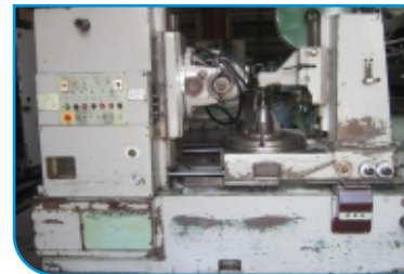
Russian Gear Hobbing E3C ø800 X 10 module with change gears
