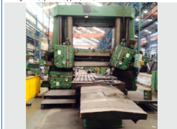
Titan Plano Miller FLP 2000 6000 x 2450mm x 2500mm with 4 Milling Heads
