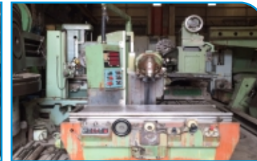
Huron Bed Milling PU601 2000 x 700mm with DRO
