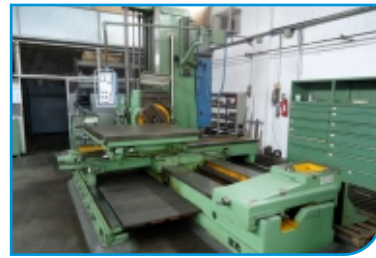
Ceruti A110 Table Type X-2200 Y-1600 with Facing Chuck, Tailstock, DRO, Angle Plates
