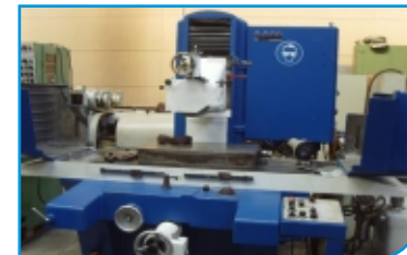
Blohm Horizontal Surface Grinding 1200mm x 500mm
