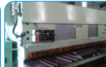
Piezok Hydraulic Shearing Machine 3100mm x 16mm
