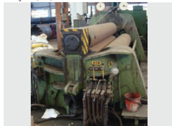
Fomp Italian Heavy Duty 4 Roll Plate Bending Machine with Pre Pinch 2600mm x 40mm
