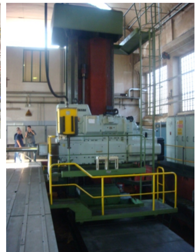
Skoda W160HA Floor Type X-8000 Y-3150 Z-1650 with DRO, Milling Head, Skoda E20 Rotary Table and floor plates YOM - 1985
