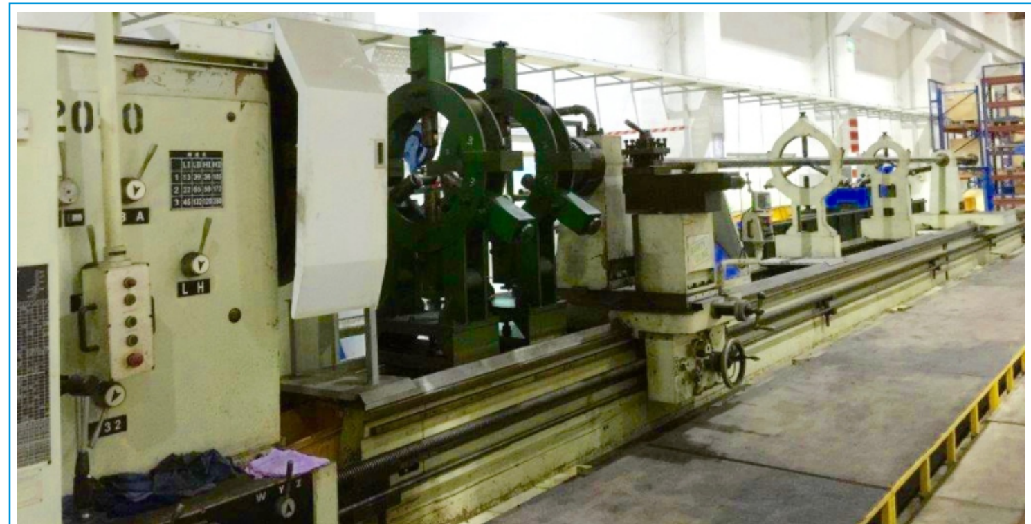
Annn Yang DY2000S Long Lathe Swing 2000mm x 15000mm Between Center With Deep Hole Drilling Attachment YOM : 2009
