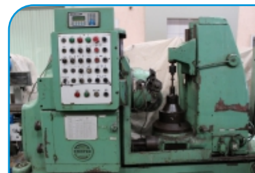
Cooper Pflauter P251 ø250mm x 6 module with Extended Tailstock
