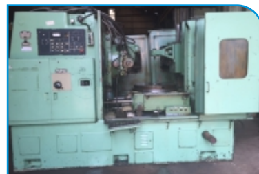
WMW FZWZ 800 Gear Hobbing ø 800 x 10 module with change gears
