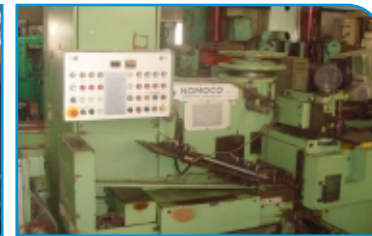
Nomoco Make VSR-4-180 Centerless Grinder ø400 x 150mm Wheel Width
