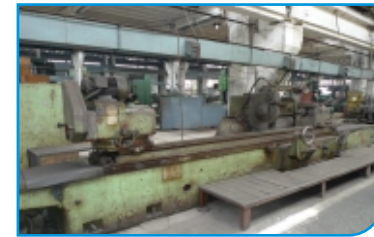
TOS BUA 63 Cylindrical Grinder ø630 X 3000mm Between Center
