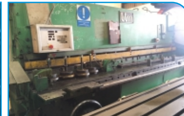
BBM Hydraulic Shearing Machine 3100mm x 6mm
