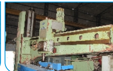
Mas VR84 – Spindle 100mm x 4000mm Arm Length
