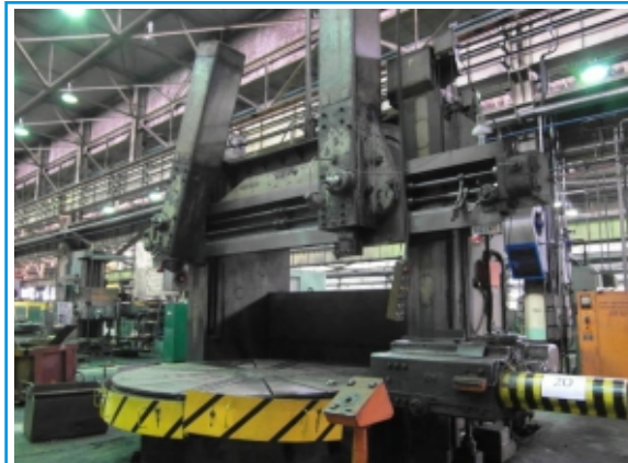
Rafamet KCF 320, Double Column VTL 3200mm Chuck, 3500mm Swing, 2100mm Height with 2 Vertical and 1 Side Tool Post
