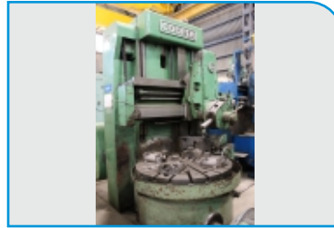
Cooper Schiess VTL 13EK125 1250mm Chuck, 1400mm Swing, 1100mm Height
