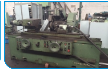
Cincinnati Cylindrical Grinder ø380mm x 900mm With Internal Grinding
