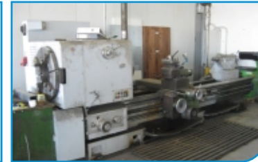
Voestaplane Oil Country lathe Spindle Bore : 360mm Between Center : 3000mm
