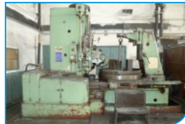
TOS FO 16 Gear Hobbing ø1600 x 16 module with attachments, change gears and work supports
