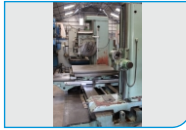
TOS W100 Table Type X-1600 Y-1200 with Facing Chuck, Tailstock, DRO, Spindle Support
