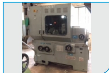
Reishauer AZA Gear Grinder YOM: 1980 with Fassler Auto Dresser ø330 x 6 module
