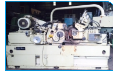
WMW SASL 200/500 Wheel ø500mm x 500mm Wheel Width
