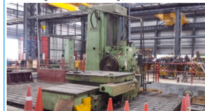
WMW BFP165/2 Floor Type X-8800 Y-2400 with DRO, Milling Head, Floor Plates, Spindle Support, WMW Rotary Table and Tailstock YOM - 1983
