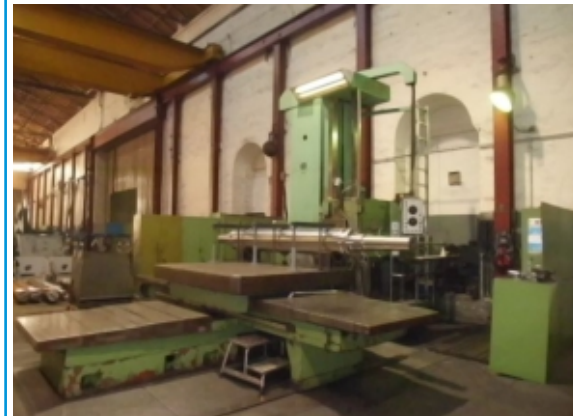
Wotan B130/150S Table Type Spindle 150mm X-2500 Y-2000 with Facing Chuck, Spindle Support, DRO, Hardened Bed
