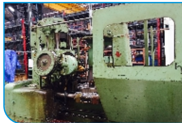
TOS FO10 Gear Hobbing ø1000 x 10 module with change gears
