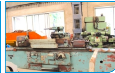
TOS BHU 32 Universal Cylindrical Grinding ø320 X 1500mm with Internal Grinding
