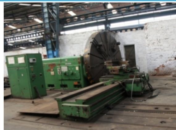
WMW Facing Lathe DP4000 Chuck 3150mm x 12000mm Between Center
