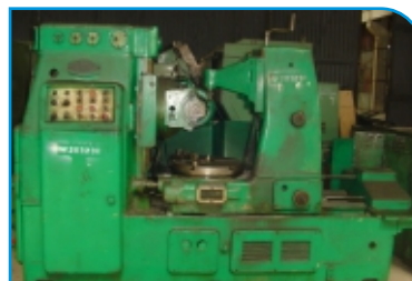
Cugir Romanian Gear Hobbing FD 320 Diameter 320 x 6 module with change gears
