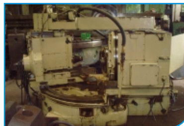
WMW Spiral Bevel Gear Generator ZFTKK 500/ 2U with cutter bodies and change gears ø500 x 12 module
