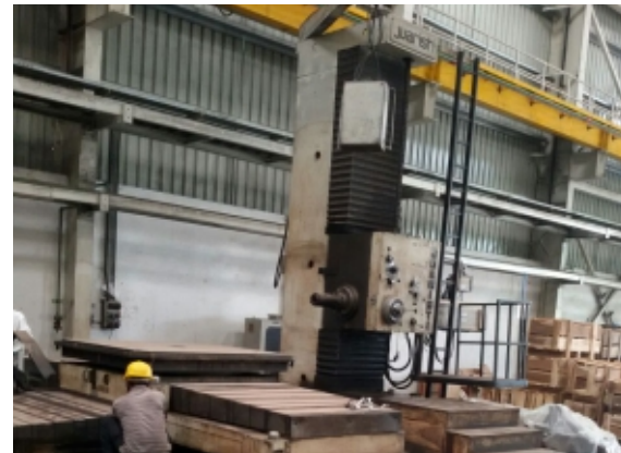
Juaristi MDR 205 CF Table Type Spindle 205mm X-2500 Y-2500 with Facing Chuck, DRO, Hardened Bed with Ball Screws YOM : 1991
