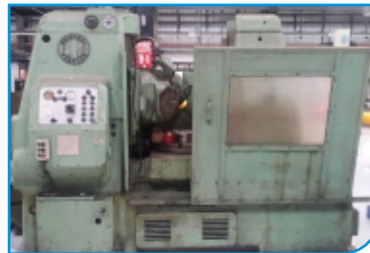
Pflauter P900 Gear Hobbing ø900 x 12 module with change gears
