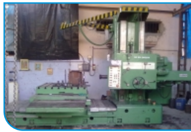
WMW BFT 110/V Table Type X-1600 Y-1200 with Facing Chuck
