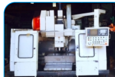
Yam VMC MV3A – Table 900 x 525mm Fanuc OM Control
