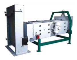
"Classifier " are used for a wide range of applications such as removing large impurities like stick, buck and leaves and are also used for removing fine dirt and sand from products in seed cleaning plants and seed processing plants.
