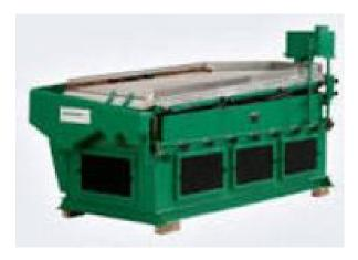
"Gravity Separator " or grain cleaner is used for separating products that are of the same size but with a difference in specific weight.
