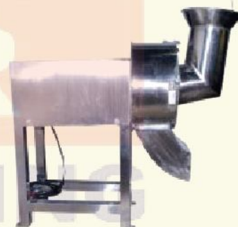
Mawa (Cold Storage) Crushing Machine
