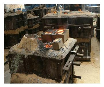
quantity of metal required for pouring. As pouring weight varies based on casting size and pressure class, a consistent rate of pouring is maintained by using the appropriate ladle to manufacture a clean casting.
