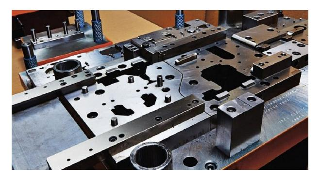
A die is a specialized machine tool used in manufacturing industries to cut and/or form material to a desired shape or profile. Stamping dies are used with a press,[1] as opposed to drawing dies (used in the manufacture of wire) and casting dies (used in molding) which are not. Like molds, dies are generally customized to the item they are used to create.
