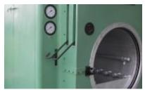
Dewaxing autoclave with inbuilt steam accumalator to take care of more steam demand during pressurisation.
