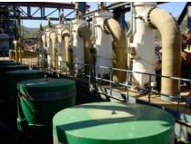
Strainers are the filters which are used for dislodging suspended solids.
