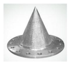
More cost effective, Conical Strainers strainer are temporary Strainers used mostly before start up of a Plant use perforated wire or mesh to trap suspended solids from a process stream. Conical strainers are usually installed horizontally in a piping system.
