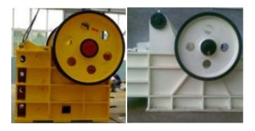
BHARATH Jaw crushers are used as primary crushers, or the first step in the process of reducing rock. They crush primarily by using compression. The rock is dropped between two rigid pieces of metal, one of which then moves inwards towards the rock, and the rock is crushed because it has a lower breaking point than the opposing metal piece. We have supplied equipment for the construction, quarry, mining, and processing industries for over 56 years, and exporting equipment for 21 years.
