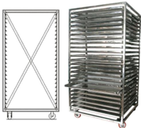
The structure for the heavy-duty Trolleys will be made from 40 mm MS angle and horizontal support will be of 25 mm angle. The design of trolley will be good enough for the proper hot air circulation. The trolley will be fitted with 2 Nos. castor wheel and 2 Nos. fixed wheel for the easy movement.
