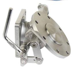
3" 45° Cleanflow Footvalve - inlet flange drilled 8 x 14mm holes equi-spaced on a 178mm PCD; outlet flange drilling as shown below. Contact parts manufactured in 316 stainless steel with Fortyt O ring to main poppet as standard.
