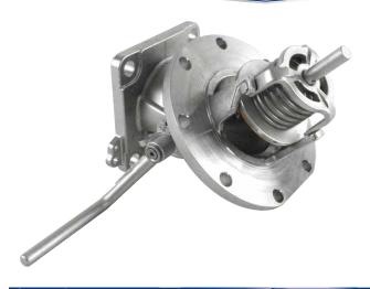
3" 45° MKIII Highlift Footvalve - inlet flange drilled 8 x 14mm holes equi-spaced on a 178mm PCD; outlet flange drilled 4 x 17mm holes on a 160mm PCD. Contact parts manufactured in 316 stainless steel with Fortyt main seal as standard.
