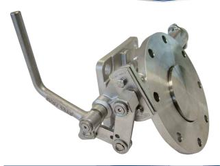
3" 30° Cleanflow Footvalve - inlet flange drilled 8 x 14mm holes equi-spaced on a 178mm PCD; square outlet flange drilled 4 x 17mm holes on a 160mm PCD. Contact parts manufactured in 316 stainless steel with Fortyt O ring to main poppet as standard.
