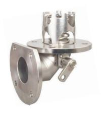
3" 90° Highlift Footvalve - inlet flange drilled 4 x 18mm holes on a 160mm PCD; outlet flange drilled 4 x 17mm holes on a 160mm PCD with flat milled at 72mm to horizontal centre line. Contact parts manufactured in 316 stainless steel with Fortyt O ring to main poppet as standard.
