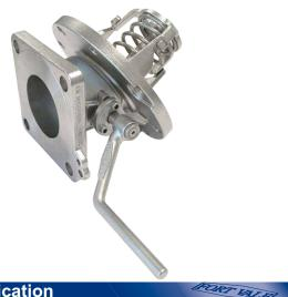
3" 30° MKIII Highlift Footvalve - inlet flange drilled 8 x 14mm holes equi-spaced on a 178mm PCD; outlet flange drilled 4 x 17mm holes equi-spaced on a 160mm PCD. Contact parts manufactured in 316 stainless steel with Fortyt O ring to main poppet as standard.
