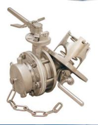
3" 45° Composite Bottom Outlet Assembly - comprising of 3" 45° Highlift Footvalve bolted through the 3" Clamped Widdop Butterfly Valve terminated with a 3" BSP eccentric outlet flange with stainless steel cap and PTFE washer. Butterfly Valve is left hand operation. Contact parts manufactured in 316 stainless steel with PTFE/Fortyt main seals.
