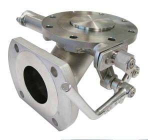
3" 90° Cleanflow Footvalve - inlet flange drilled 8 x 14mm holes equi-spaced on a 178mm PCD; outlet flange drilled 4 x 17mm holes equi-spaced on a 160mm PCD with flats milled top and bottom. Contact parts manufactured in 316 stainless steel with Fortyt O ring to main poppet as standard.
