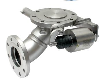
4" 90° Pneumatic Cleanflow Footvalve - inlet flange drilled 8 x 18mm holes equi-spaced on a 210mm PCD (DIN125 PN16); outlet flange drilled 8 x 18mm holes equi-spaced on a 180mm PCD (DIN100 PN16). Contact parts manufactured in 316 stainless steel with Fortyt O ring to main poppet as standard.
