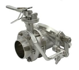
3" 45° Composite Bottom Outlet Assembly - comprising of 3" Cleanflow Footvalve bolted through the 3" Clamped Butterfly valve terminated with a 3" BSP outlet flange. Butterfly valve is left hand operation. Contact parts manufactured in 316 stainless steel with Fortyt main seal to footvalve and PTFE main seal to butterfly valve.
